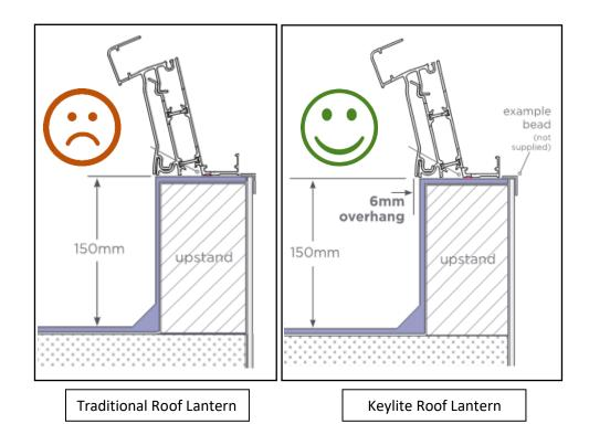
It is imperative that the 6mm overhang is adhered to, as were the Keylite Flat Roof Lantern to be installed square to the upstand and this silicone seal applied then the built in drainage channels would be blocked and any water as a result of naturally forming condensation would build up inside the unit as it physically has nowhere else to go.
