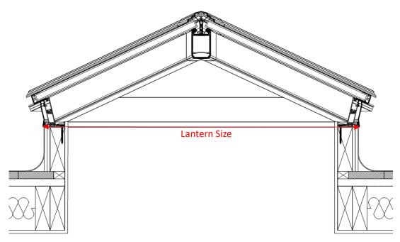
Keylite require there to be a 6mm overhang of the lantern frame on the upstand all the way around the perimeter of the lantern. See below;
