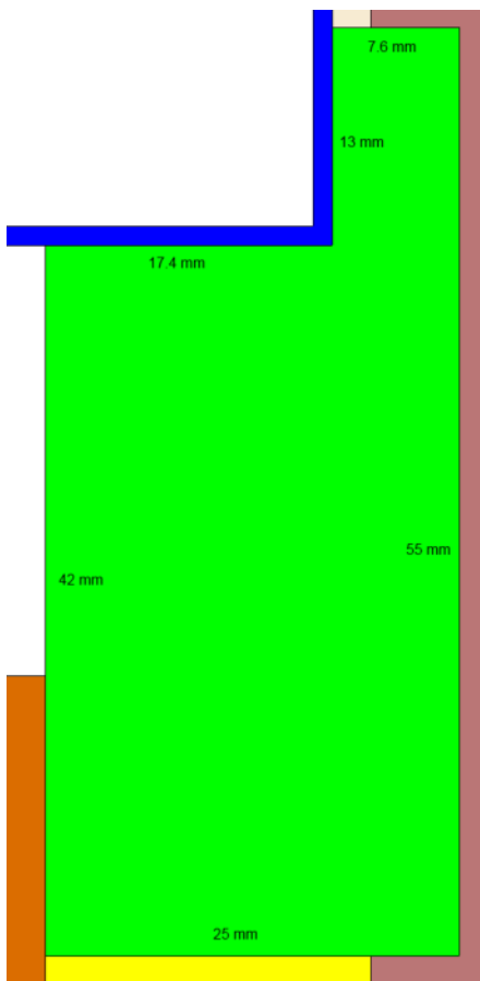
Figure 6. An expanded view of the thermal collar, showing the dimensions of the collar in mm. This figure refers to the left collar, however the right collar has the same dimensions and is a mirror image of the left collar.
