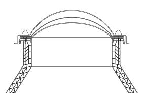
High Security Screw Bolt Triple Glazed Polycarbonate Dome
