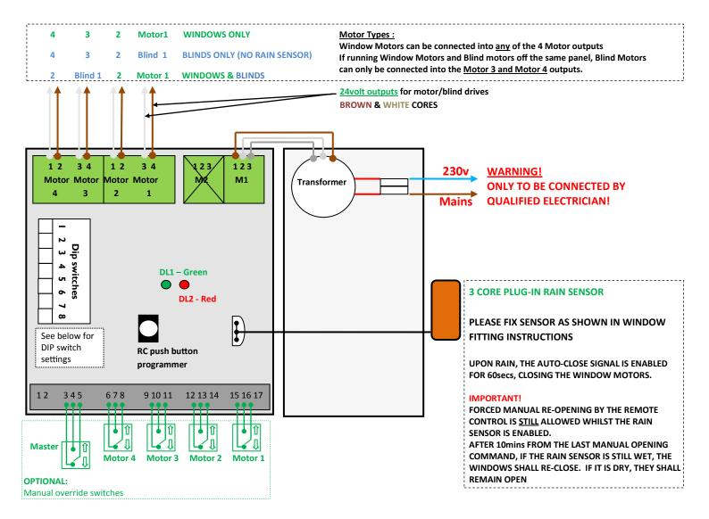
The TF24R control panel can be used for a range of different operations, from operating 1 electric window and/or electric blind to 4 windows or 4 blinds.
